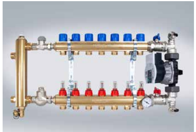
Control manifold HCM-DR with high-efficiency pump and thermoseparator, version 2.0, 2-9 heating circuits 1" IT or 10-16 heating circuits 5/4"
